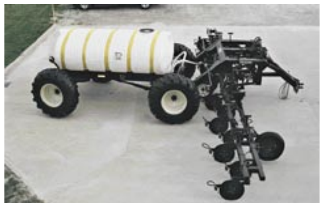
The toolbar hitch attaches to the front of the All Steer High Capacity Cart after the pull hitch is removed.
