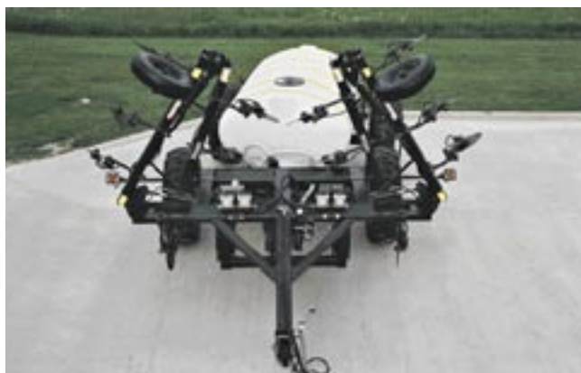
The 16-row All Steer Plus Fertilizer Toolbar folds twice and has a transport width of 17 feet.
