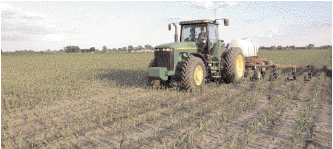
When sidedressing, John Blacksmith of Argyle, Iowa, pulls a 1,000-gallon tank mounted on a wagon running gear that straddles four rows for stability.
