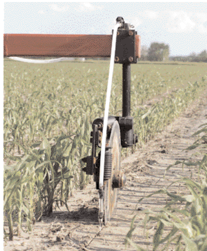
A solid-stream nozzle shoots a stream of 32% nitrogen into the slot made by a smooth coulter.
