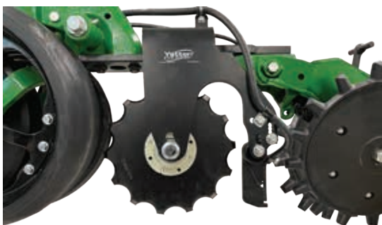
Single wheel with 2968-090 Spring-Loaded Knife option
