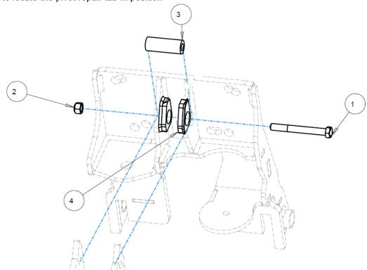
Step 2: Weld in pivot repair tabs. Paint after surface has cooled.
