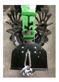
**Adjustments:** Position brackets to carry front of chain about 3" to 4" above soil. Securely tighten hardware. For best soil leveling, keep front end of the chain as low as possible while maintaining clearance above the soil for the bracket ends. Use drag chains when planting in minimum till or in no-till where at least some of the soil surface is dry. Lift the chain into storage position when conditions aren't desirable to operate the drag chain.
