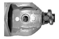
STEP 5. SECURELY TIGHTEN 12 MM BOLT.
