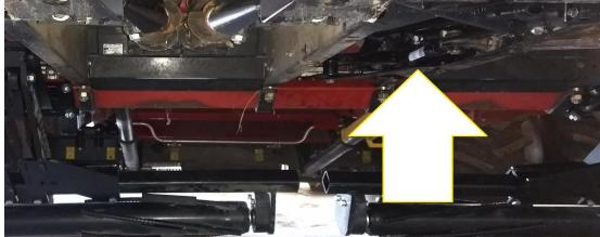
**Step 1:** Attach the 5000-260 mount brackets to the frame using 5/8" X 6 bolts, clamp straps, & 5/8" lock hex nuts. 4408 Folding corn heads will use 4) 5000-288 double mount brackets. Between rows 1-2 & 7-8, 5000-460 spacer blocks, 5/8" X 8" bolts will be used. Mounts between rows 3-4 & 5-6 will not use spacer blocks & will use 5/8" X 6" bolts.
