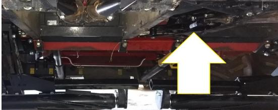
Step 1: Attach the 5000-260 mount brackets to the frame using 5/8" X 6 bolts, clamp straps, & 5/8" lock hex nuts. 4408 Folding corn heads will use 4) 5000-288 double mount brackets. Between rows 1-2 & 7-8, 5000-460 spacer blocks, 5/8" X 8" bolts will be used. Mounts between rows 3-4 & 5-6 will not use spacer blocks & will use 5/8" X 6" bolts.
