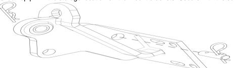
**Step 3:** Attach the pivot arms to the mount brackets using the 5/8 X 3 bolts, pivot bushings, & lock hex nuts. Fully tighten all hardware. **NOTE:** Make sure the pivot arm orientation matches the diagrams below.
