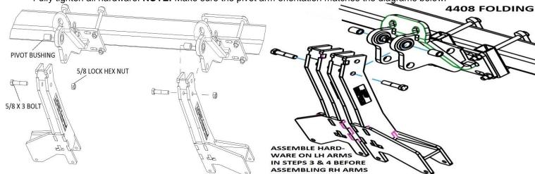
**Step 4:** Install the pushrods into the mount brackets. Then, attach to the pivot arms with the 5/8 shoulder bolts, washers, & ½ jam lock hex nuts. Now install the compression spring, spring bushing, and ¾ lock hex nuts. **Note:** The washers are installed on each side of the "eye" of the pushrod.
