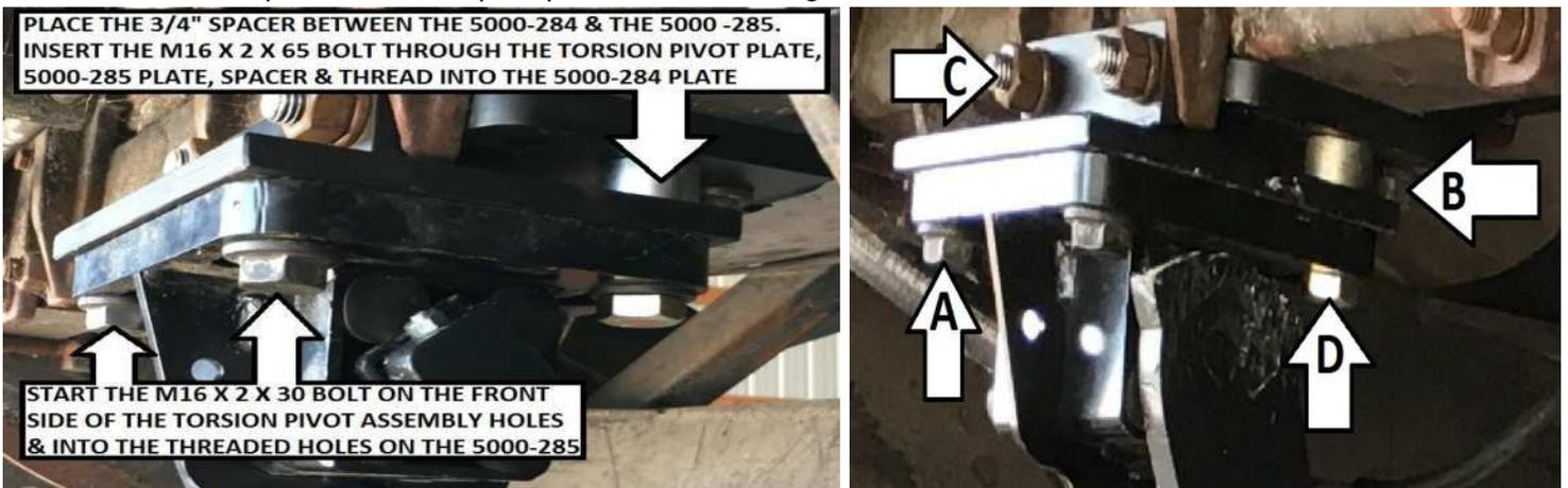
**Step 3:** Refer to page 14 for instructions on installing the 5000-292 torsion arm.
