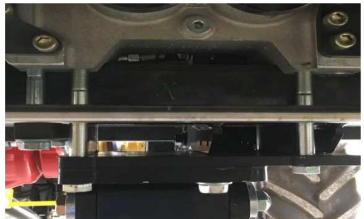
1 SET OF GEAR BOX MOUNTING BOLTS REMOVED
