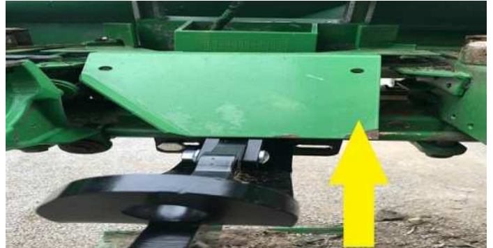
MOUNTING BRACKET ASSEMBLY INSTRUCTIONS (ROW 2-3 AND 10-11) JD 1293 (12 ROW) CORN HEAD (ONLY)
