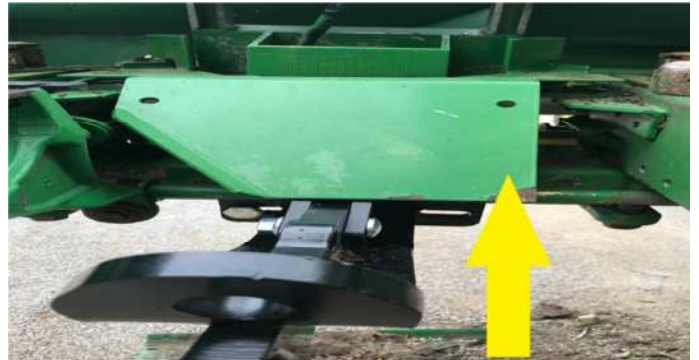
MOUNTING BRACKET ASSEMBLY INSTRUCTIONS (ROW 1-2 AND 7-8) JD 893 (8 ROW) CORN HEAD (ONLY)
