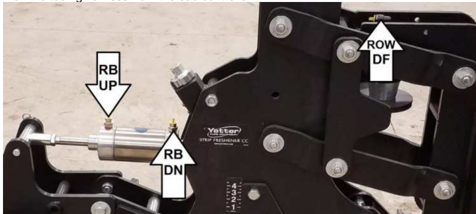
BELOW IS AN EXAMPLE OF HOW TO ROUTE THE AIRLINE FROM THE TOOLBAR TO EACH FUNCTION. ZIP TIE THE AIRLINE NEATLY & OUT OF HARMS WAY WHEN IN USE & FOLDING/UNFOLDING MACHINE
