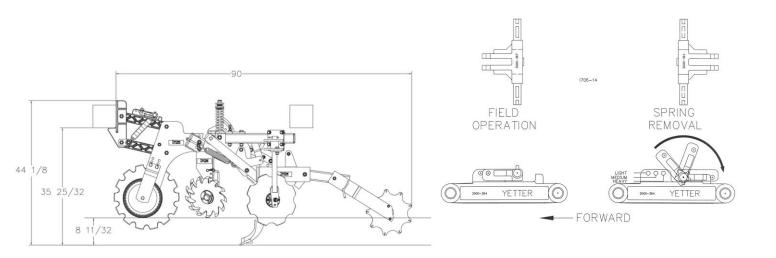
**STEP 1.** Disengage Rolling Basket Attachment – Lift basket and insert pin. See diagram.
