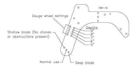
STEP 3. Set the depth of the knife by adjusting toolbar height and spring tension on the parallel arms.
