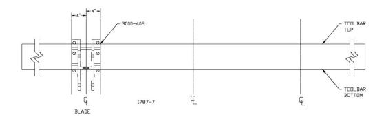
**STEP 2.** Centering on each row, attach the (3000-149) parallel arm assembly to the toolbar with the appropriate <sup>3</sup>/<sub>4</sub>" u-bolts, lock washers and hex nuts. Torque the u-bolts to 200 ft. lbs. *Recheck the torque after 10 hours of use.*
