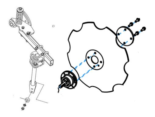
**STEP 4:** Adjust the angle of the disc blades so they are centered on the knife, and within the starting parameters shown below
