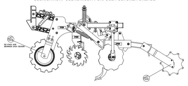
To ensure longevity and reliability of the MAVERICK OPENER HR Plus, the recommended lubrication schedule should be followed using multi-purpose grease at intervals as indicated.
