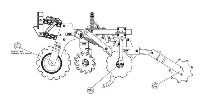
To ensure longevity and reliability of the MAVERICK OPENER™ HR Plus, the recommended lubrication schedule should be followed using multi-purpose grease at intervals as indicated.
