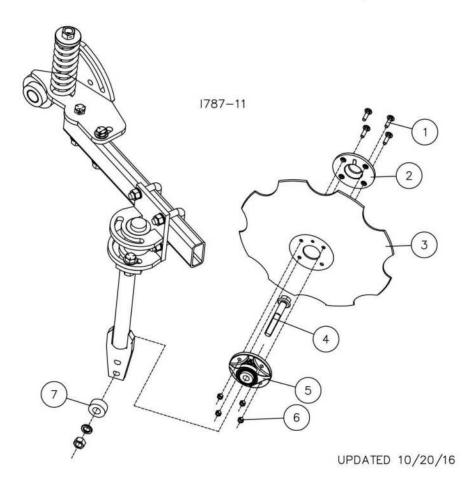
**STEP 4:** Adjust the angle of the disc blades so they are centered on the knife, and within the starting parameters shown below
