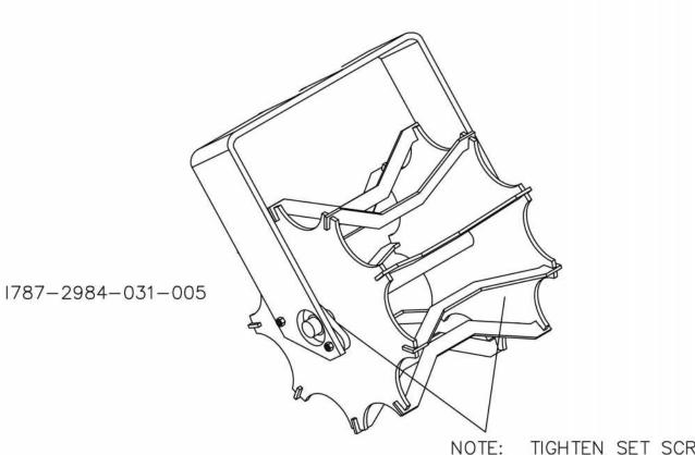
TIGHTEN SET SCREWS IN BEARINGS AFTER THE UNIT IS COMPLETELY ASSEMBLED, MAKE SURE BASKET IS CENTERED.
