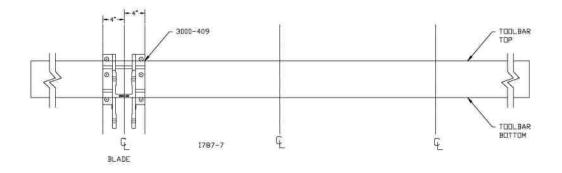
**STEP 2.** Centering on each row, attach the (3000-149) parallel arm assembly to the toolbar with the appropriate <sup>3</sup>/<sub>4</sub>" u-bolts, lock washers and hex nuts. Torque the u-bolts to 200 ft. lbs. <u>*Recheck the torque after 10 hours of use.*</u>
