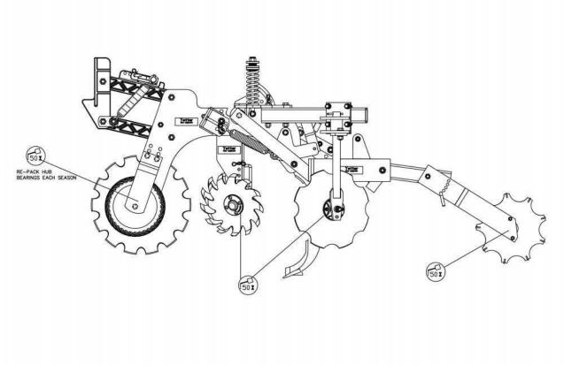
To ensure longevity and reliability of the MAVERICK OPENER HR Plus, the recommended lubrication schedule should be followed using multi-purpose grease at intervals as indicated.
