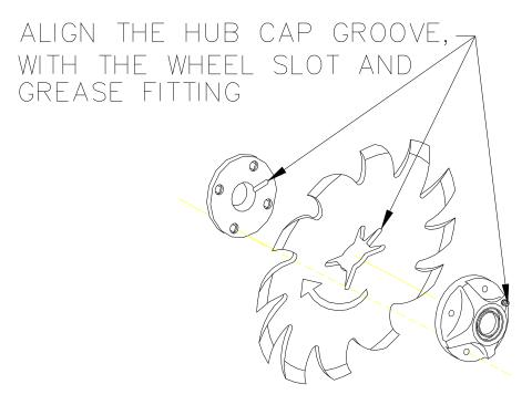
**NOTE:** Be certain to align the grease fitting with the slot in the wheel and the hubcap so that the grease can flow freely.
