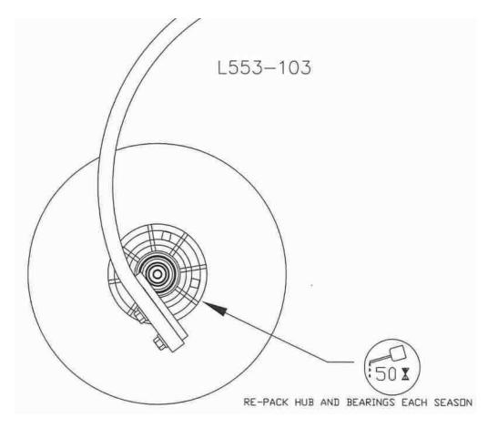
To ensure longevity and reliability of the V.T.A.™ Coulter, the recommended lubrication schedule should be followed using multi-purpose grease at hourly intervals as indicated.
