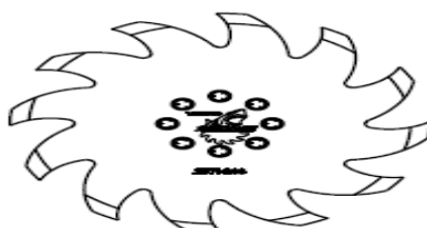
SHARKTOOTH WHEEL ASSEMBLY RIGHT HAND 2966-140-ST(SHOWN) LEFT HAND 2966-141-ST
