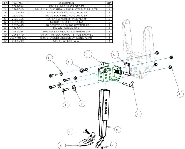
**STEP 2 Continued:** For the 2965-028, install the mount bracket assembly (2967-195). At this time tighten the mounting hardware.
