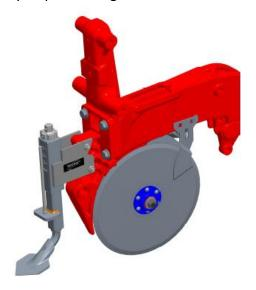
step 2 Continued: For all other row units attach using three ½" bolts and locknuts. NOTE: put two bolts in the top mounting holes, and the smaller flat washer (2526-355) under the head of the bolt. Put a single bolt in one of the bottom holes with the larger flat washer (2526-402) under the head of the bolt. NOTE: the side with which the bottom bolt is installed will vary depending on planter model.
