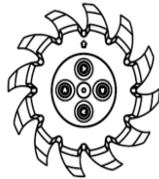
SHARKTOOTH WHEEL ASS'Y W/POLY FLOATER WHEEL RIGHT HAND 2966-140-ST-PFW(SHOWN) LEFT HAND 2966-141-ST-PFW
