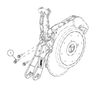
STEP 2. Install the 2966-021 residue manager onto the 2960 coulter using the  $5/8" \times 2"$  bolts, 5/8" washers, bushings and flange hex nuts.
