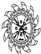
SHARKTOOTH WITH FLOATER WHEEL ASSEMBLY RH - 2966-140-ST-FW (SHOWN) LH - 2966-141-ST-FW
