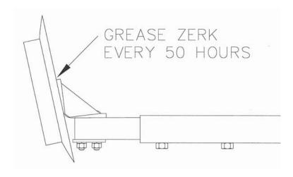
IMPORTANT: The recommended service intervals are based on normal conditions; severe or unusual conditions may require more frequent lubrication.
