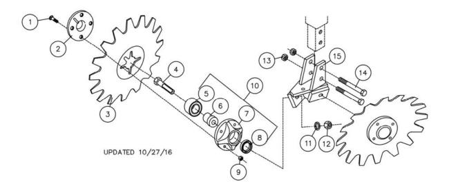
2967-093-R (SHOWN) 2967-093-L MULTI-NOTCHED DISC SCREW ADJUST R.M., RH (SHOWN) MULTI-NOTCHED DISC SCREW ADJUST R.M., LH
