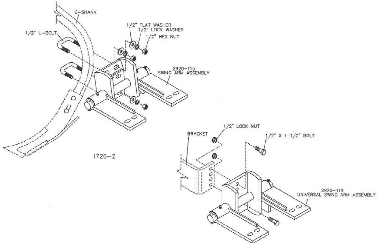
**STEP 2.** Attach the 2920-117 Arm Hub Assembly to the 2920-115 Swing Arm using the 1/2" carriage bolts, flat washers, lock washers and hex nuts.
