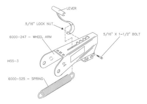
**STEP 5.** First, hook the spring onto the 6200-202 – close wheel mount then attach the close wheel arm assembly to the left hand side of the 6200-202 close wheel mount and the row unit using the  $\frac{1}{2}$ " x 1" bolt, 6200-441 – link and lock nut. Insert the 6000-523 – eccentric bushing into the close wheel arm and connect the close wheel arm to the 6200-441 - link and 6200-202 – wheel mount using a  $\frac{1}{2}$ " x 2-1/2" bolt,  $\frac{1}{2}$ " flat washer and lock nut.
