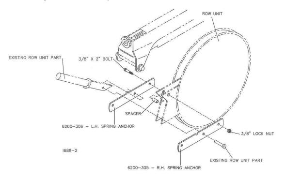
**STEP 3.** Attach the 6200-202 – v-closing wheel mount to the spring anchor straps using a 3/8" x 1-1/2" bolt, 3/8" flat washer, spacer, 3/8" flat washer and lock nut.
