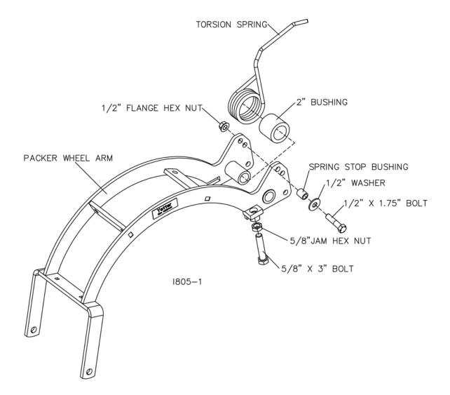
STEP 4. Attach the packer wheel arm assembly to the mount bracket.
