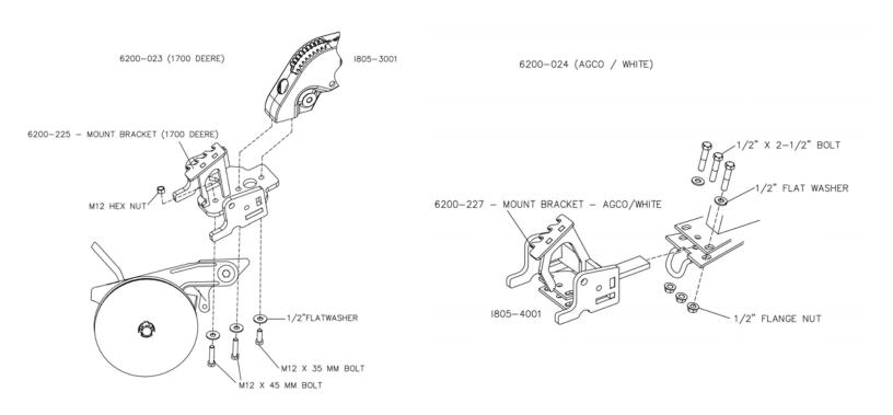
STEP 2. Attach the v-closing wheel assembly to the packer wheel mount bracket.  $1 \times 12$  are not shown for clarity of illustrations,  $1 \times 12$  wheels are intended to be used with the 6200 packer wheel.
