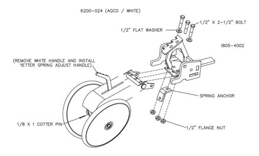
STEP 3. Attach the spring stop, spring and height adjustment to the packer wheel arm.
