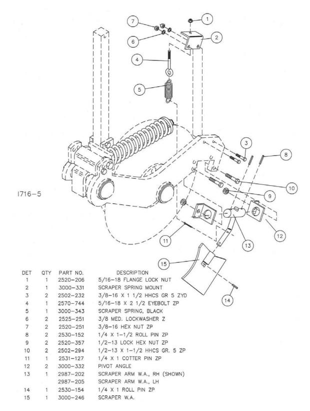
3000-048-L - 16 SPRING LOADED LIQ SIDE KNIFE ASSY, LH 3000-048-R - 16 SPRING LOADED LIQ SIDE KNIFE ASSY, RH 3000-049-L - 16 SPRING LOADED DRY SIDE KNIFE ASSY, LH 3000-049-R - 16 SPRING LOAD DRY SIDE KNIFE ASSY, RH
