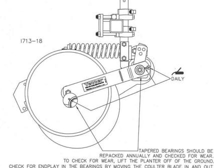
TO CHECK FOR WEAR, LIFT THE PLANTER OFF OF THE GROUND. CHECK FOR ENDPLAY IN THE BEARINGS BY MOVING THE COULTER BLADE IN AND OUT. ROTATE THE BLADE TO CHECK FOR ROUGHNESS IN THE BEARINGS. IF BEARINGS SOUND ROUGH, THE HUB SHOULD BE REMOVED AND THE BEARINGS INSPECTED AND REPLACED IF NECESSARY.
