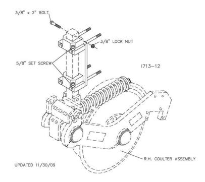
**STEP 4.** Attach the coulter/shank/clamp assembly to the fertilizer toolbar using the 3000-301 wedge, clamp plate and ½" lock nuts.
