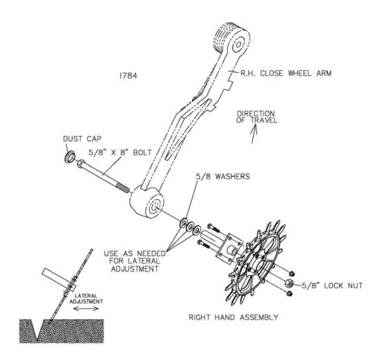
Lateral adjustment is important because the seed furrow may not be <u>covered/closed</u> if the closing wheel is <u>too far</u> from the seed furrow; or the <u>seed placement</u> will be effected if the close wheel is <u>too close</u> to the seed furrow.
