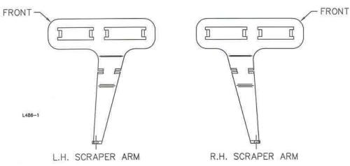
1. Determine R.H. and L.H. scraper arms using illustration below. Note: tabs are pointing down.
