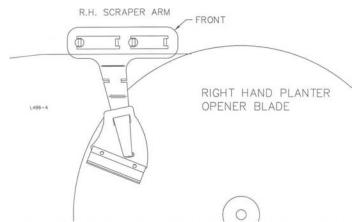
Release scraper arm, spring tension will hold the scraper against the planter disc blade.
