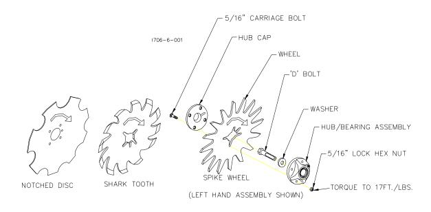
**IMPORTANT**: THE 2527-530 WASHER MUST BE INSTALLED OR THE WHEEL AND HUB ASSEMBLY WILL FALL OFF DURING USE.
