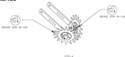
IMPORTANT: The recommended service intervals are based on normal conditions; severe or unusual conditions may require more frequent lubrication.
