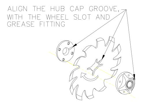
**NOTE:** Be certain to align the grease fitting with the slot in the wheel and the hubcap so that the grease can flow freely.
