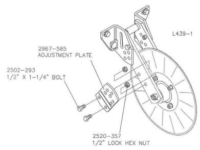
2. Remove the  $\frac{1}{2}$ " x 5" bolt which attaches the coulter arms to the mounting brackets through the slot. Save the  $\frac{1}{2}$ " lock nut and the  $\frac{1}{2}$ " flat washers for later use.
