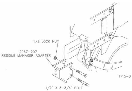
STEP 1. Attach the 2967-297 residue manager adapter to the planter using the 2) ½" x 3-3/4" bolts and lock nuts.
