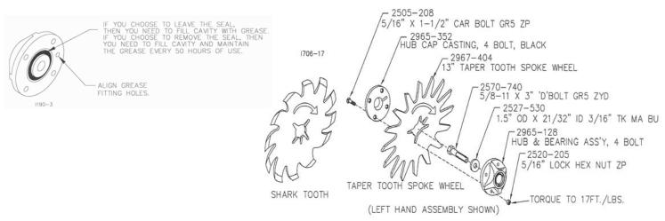
IMPORTANT: <u>2527-530 Washers</u> must be installed or Residue Manager Wheel and hub assembly will fall off during use.
