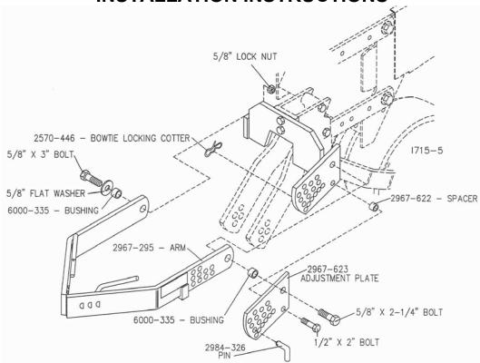
**STEP 3.** Attach the 2967-295 arm to the 2967-296 mount bracket using the 5/8" bolts, flat washers, bushings, 2967-623 adjustment plate and 5/8" lock nuts. Also, install the  $\frac{1}{2}$ " x 2" bolt, 2967-622 spacer,  $\frac{1}{2}$ " lock nut, 2984-326 pin and 2570-446 bowtie cotter on the 2967-623 adjustment plate.
