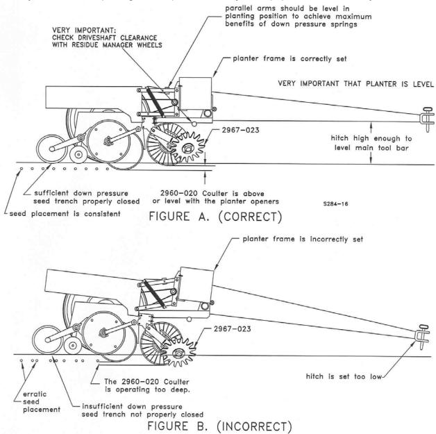
**Figure A. –** The planter hitch and frame are both 20" off the ground. To ensure this, visually check to see that the planter boxes are level and that the planter unit parallel arms are also parallel with the ground. **When using planter attachments located in front of the planter unit, this setting is very important.**
