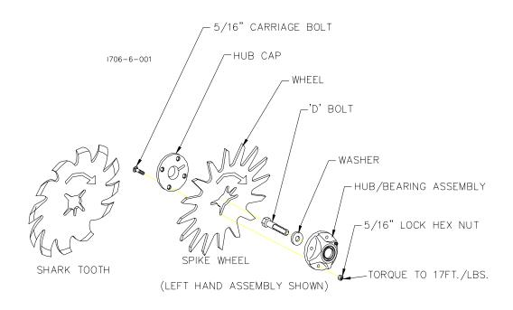
**IMPORTANT**: THE 2527-530 WASHER MUST BE INSTALLED OR THE WHEEL AND HUB ASSEMBLY WILL FALL OFF DURING USE.
