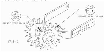
IMPORTANT: The recommended service intervals are based on normal conditions; severe or unusual conditions may require more frequent lubrication.
