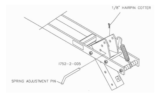
USE THE LIGHTEST SPRING PRESSURE THAT WILL PROVIDE A SATISFACTORY BERM. ATTACH THE BASKET MOUNT BRACKET TO THE PIVOT BRACKET USING THE 5/8" X 4 ½" HEX BOLT AND 5/8" LOCK HEX NUT. ALSO, INSTALL THE ADJUSTMENT PIN AND 1/8" HAIRPIN COTTER.
