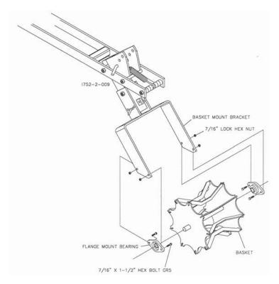
CENTER THE BASKET IN THE BASKET MOUNT BRACKET AND "TRIPLE TIGHTEN" THE SET SCREWS.
