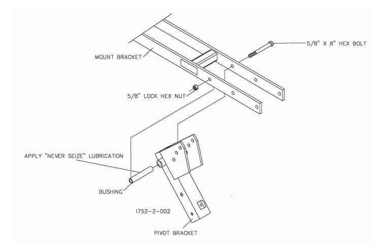
LIFT THE PIVOT BRACKET AND INSTALL THE 5/8" X 8" HEX BOLT AND 5/8" LOCK HEX NUT.
