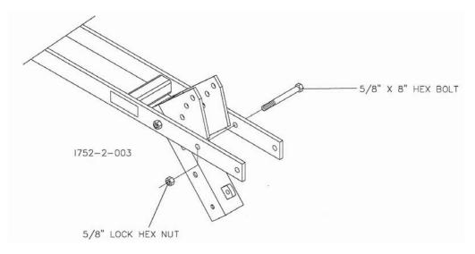
ATTACH THE EXTENSION SPRING TO THE MOUNT BRACKET. USE THE 5/8" X 8" HEX BOLT, (6) <sup>3</sup>/<sub>4</sub>" SPACERS AND 5/8" LOCK HEX NUT.
