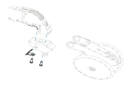
STEP 3. INSERT THE 12MM BOLT THROUGH THE 2570-790 WHEEL STOP MOUNTING HOLE AND THREAD IT BY HAND BACK INTO THE ROW UNIT.
