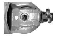
STEP 5. SECURELY TIGHTEN 12 MM BOLT.
