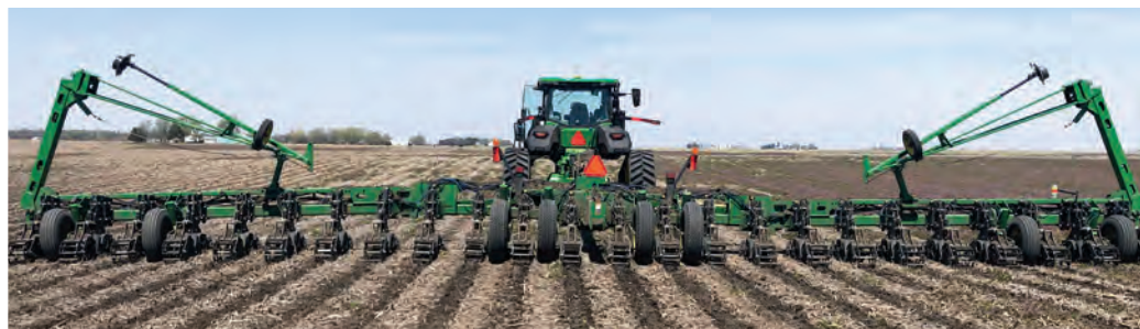
Shown with row cleaner, Poly Floater Wheel, Air Assist Cylinder, and depth control options
