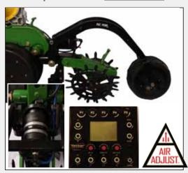
The Air Adjust system (bottom left) allows for precise adjustments to be made from the controller in the tractor cab (bottom middle), making it convenient to change settings for different conditions.
