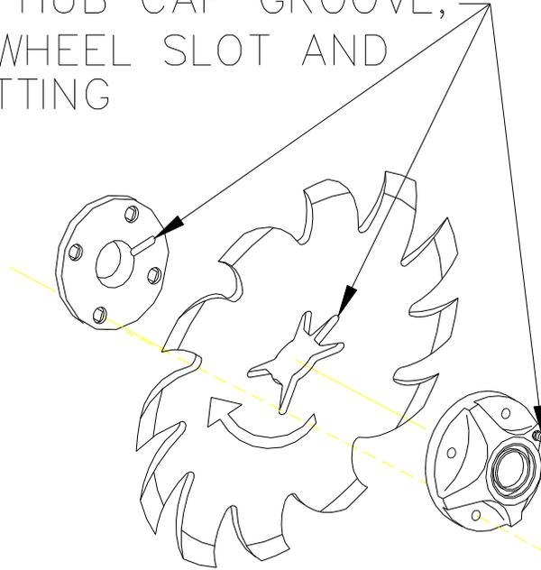
**NOTE:** Be certain to align the grease fitting with the slot in the wheel and the hubcap so that the grease can flow freely.
