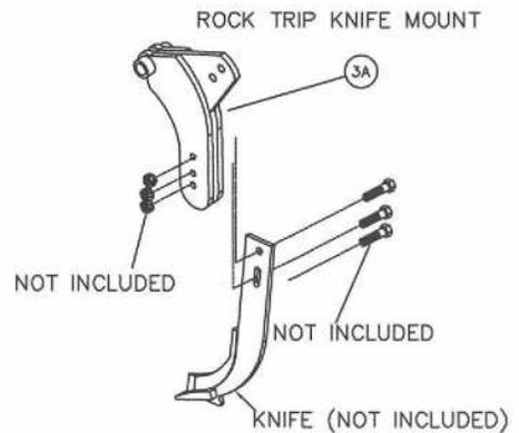
**STEP 4.** Tighten all bolts to recommended torques from the table of this manual, unless the torque is otherwise specified.
