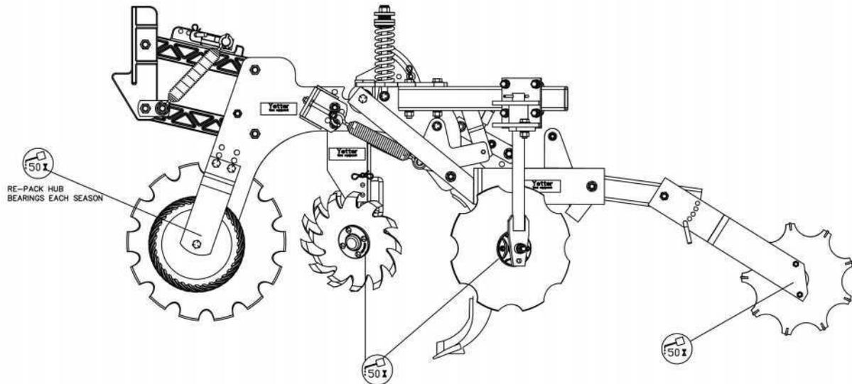
To ensure longevity and reliability of the MAVERICK OPENER<sup>®</sup> HR Plus, the recommended lubrication schedule should be followed using multi-purpose grease at intervals as indicated.
