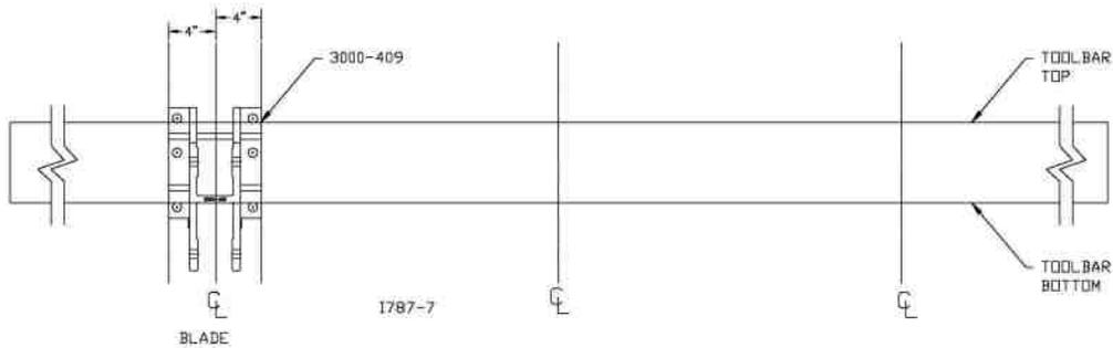
**STEP 2.** Centering on each row, attach the (3000-149) parallel arm assembly to the toolbar with the appropriate 3/4" u-bolts, lock washers and hex nuts. **Recheck the torque after 10 hours of use.**
