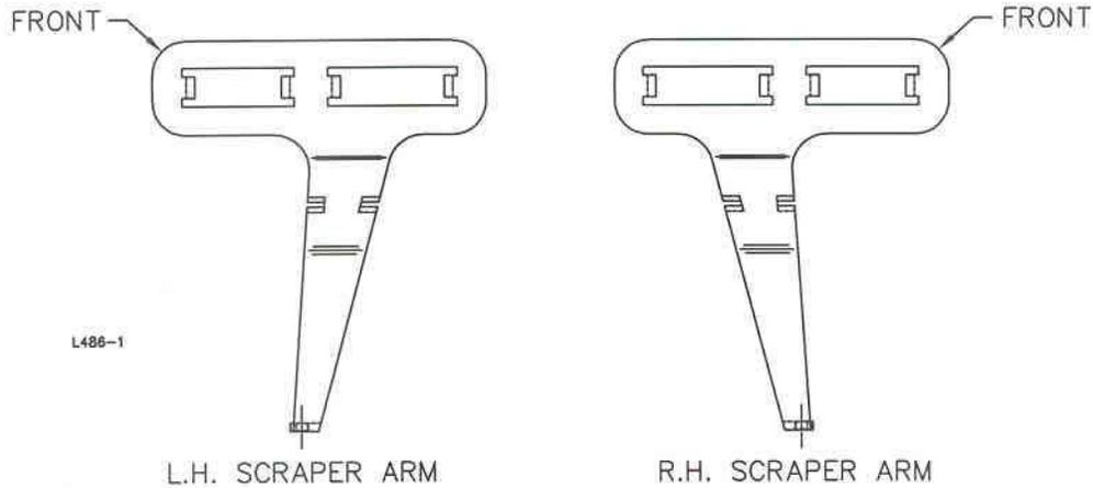
2. Mounting tabs that are not going to be used (based upon the model of planting unit to be mounted on) need to be bent flush with the scraper arm or removed from the scraper arm.
