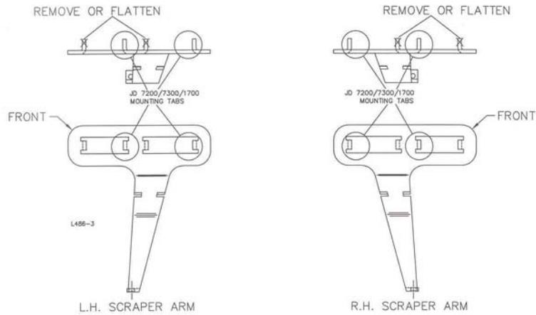
3. Assemble the right and left scraper arms with the spring hooked into the arm slots.
