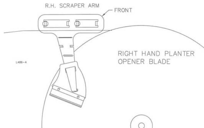
7. Release scraper arm, spring tension will hold the scraper against the planter disc blade.
