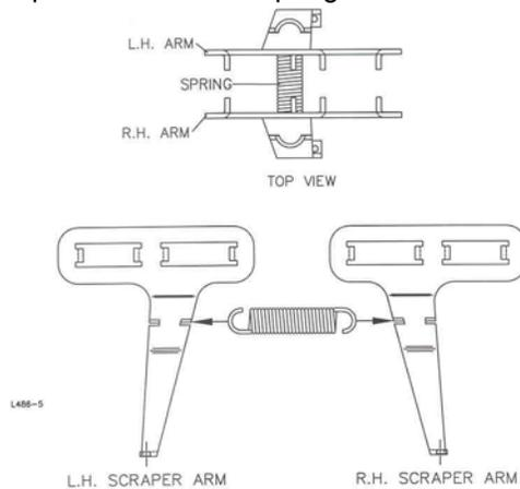
4. Place the tabs of one arm into the mounting holes and pull the assembly under the planter opener frame to the other side and insert the tabs into the mounting holes. Note: check to make sure the tabs are securely inserted in the scraper mounting holes.
