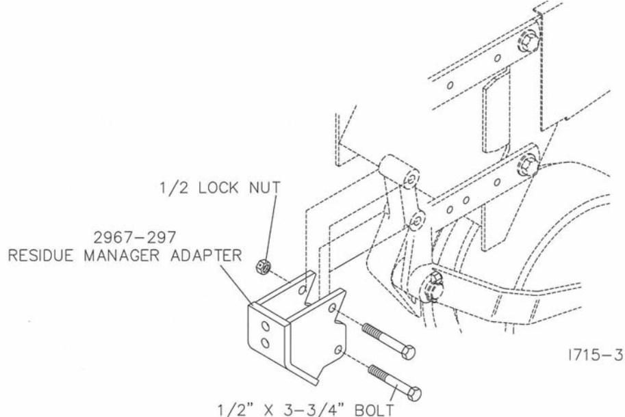
**STEP 1.** Attach the 2967-297 residue manager adapter to the planter using the 2)  $\frac{1}{2}$ " x 3- $\frac{3}{4}$ " bolts and lock nuts.
