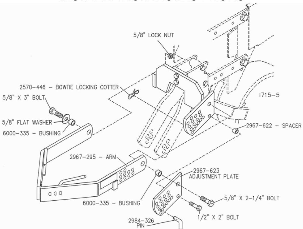
**STEP 3.** Attach the 2967-295 arm to the 2967-296 mount bracket using the 5/8" bolts, flat washers, bushings, 2967-623 adjustment plate and 5/8" lock nuts. Also, install the 1/2" x 2" bolt, 2967-622 spacer, 1/2" lock nut, 2984-326 pin and 2570-446 bowtie cotter on the 2967-623 adjustment plate.
