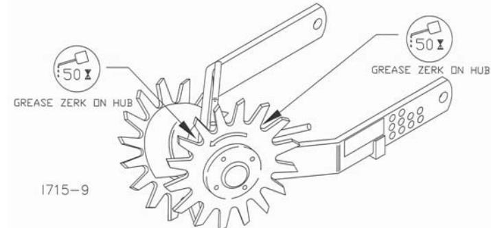
**IMPORTANT: The recommended service intervals are based on normal conditions; severe or unusual conditions may require more frequent lubrication.**
