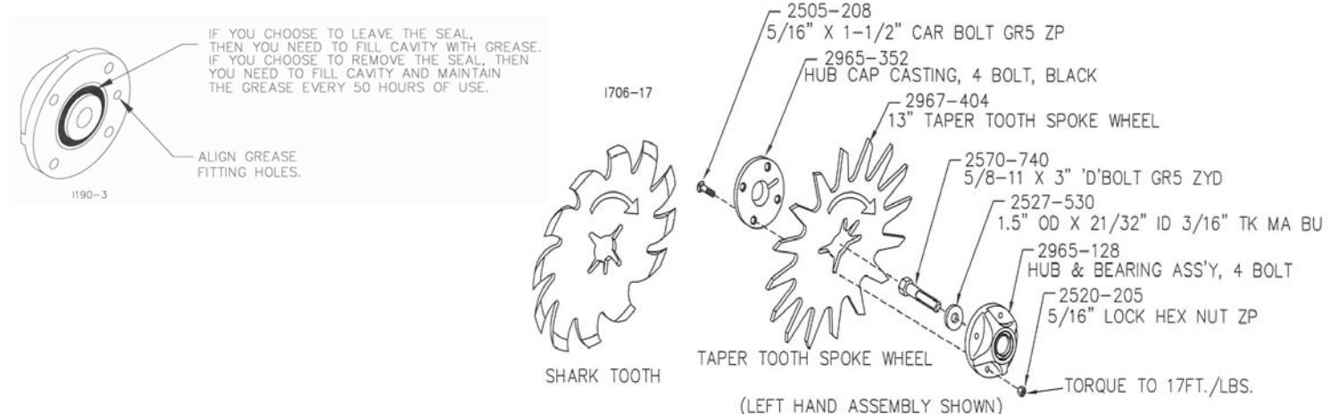
**IMPORTANT:** 2527-530 Washers must be installed or Residue Manager Wheel and hub assembly will fall off during use.
