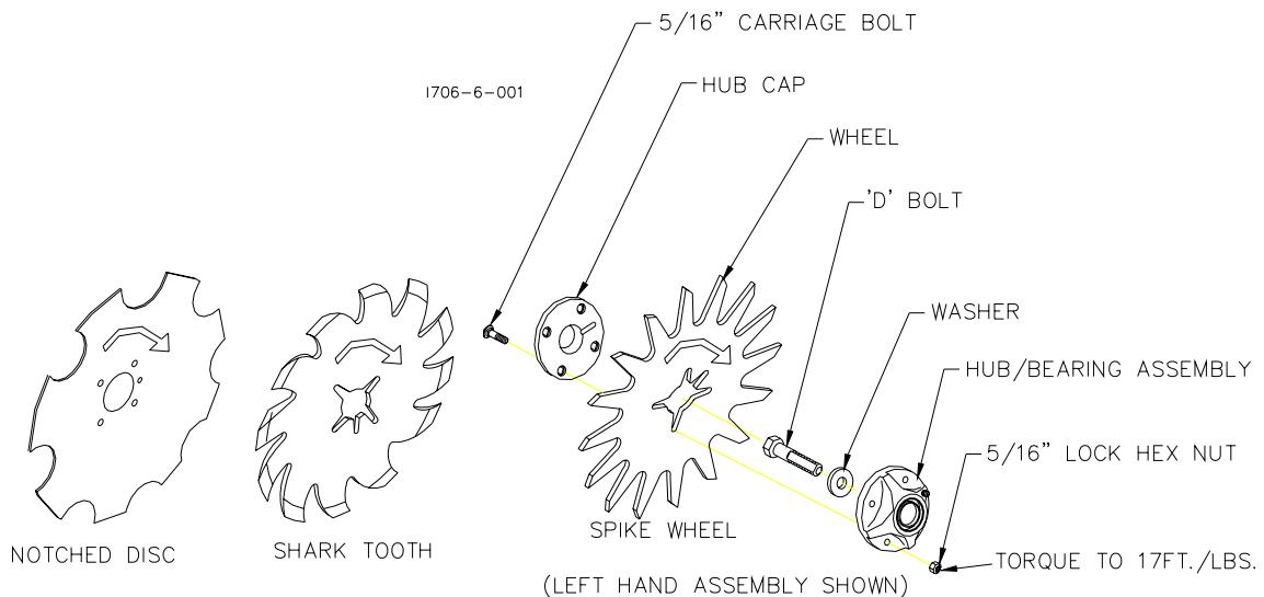
**IMPORTANT:** THE 2527-530 WASHER MUST BE INSTALLED OR THE WHEEL AND HUB ASSEMBLY WILL FALL OFF DURING USE.
