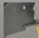
The spring-loaded knife with carbide insert extends wear and life between replacements.
