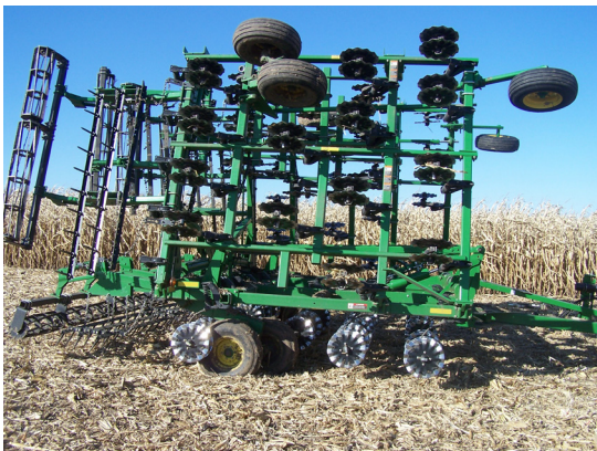
Vertical tillage machines have become quite popular on many farms. Some operations have chosen to adapt vertical tillage attachments for existing chisel plows or field cultivators to drastically reduce the cost of getting into this practice.
