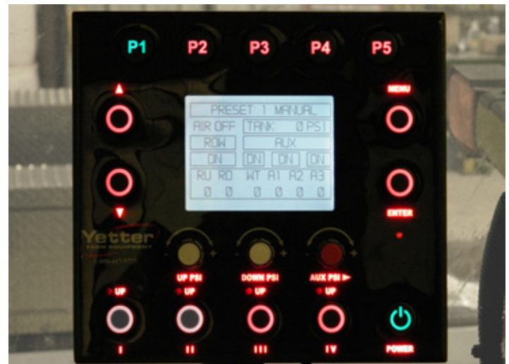
The 2940 Air Adjust Residue Manager conveniently adjusts planter attachments from the cab. Push the up button to raise for wet spots or waterways. Pictured is the In-Cab Controller.
