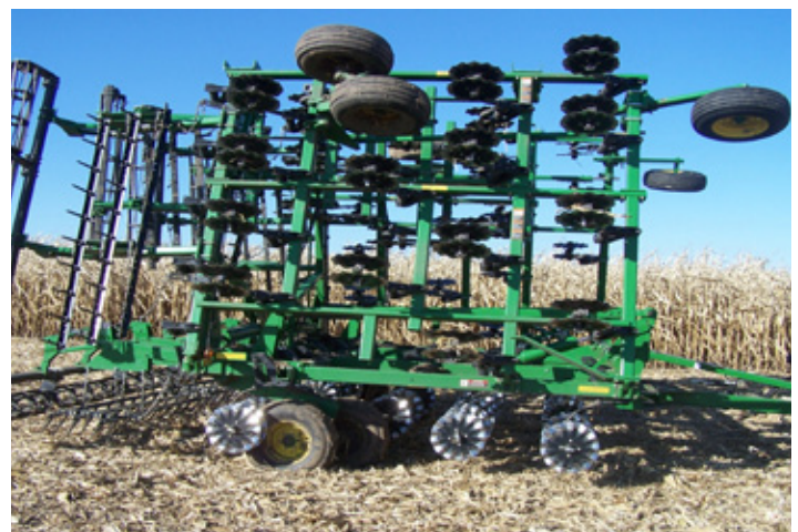
Vertical tillage tools like the Yetter Vertical Tillage Attachment can allow you to start planting sooner by facilitating soil warm-up.
