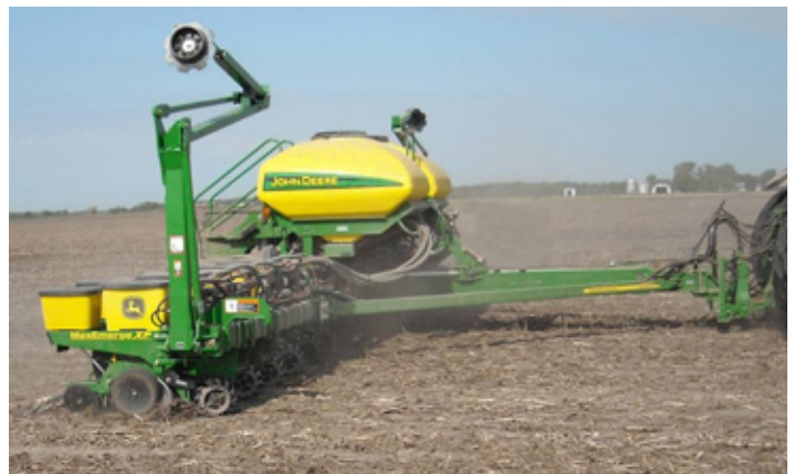
Levelness of the planter is crucial to ensure it will work properly.
