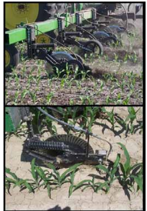
Side-dressing efficiently places nitrogen when the crop needs it most—either anhydrous application (top) or liquid application (bottom) are options.
