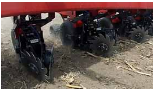
Air adjust residue managers, such as the Yetter 2940 for Case, and other new technology have allowed farmers to make adjustments from the cab with a touch of the button.
