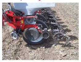
Proper planter attachments, like Yetter SharkTooth® residue managers and spike closing wheels, are essential to proper planting into cover crops.
